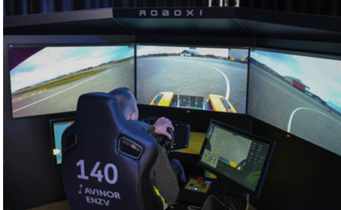
Remotely driving Roboxi at Sola Airport with low latency.
