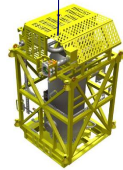
Scrubber Weight: 211 tons Size: 8 x 8 x 12 m
