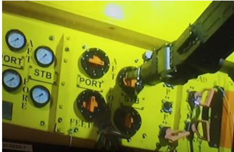
2 ROV panel for release of lifting frame
