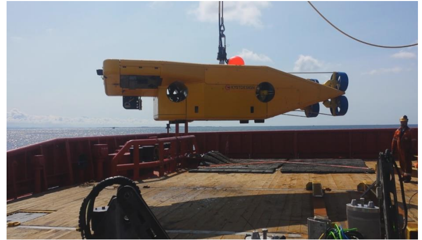
SUPERIOR ROV WITH SKID REMOVED FOR SEABED MAPPING SURVEYS
