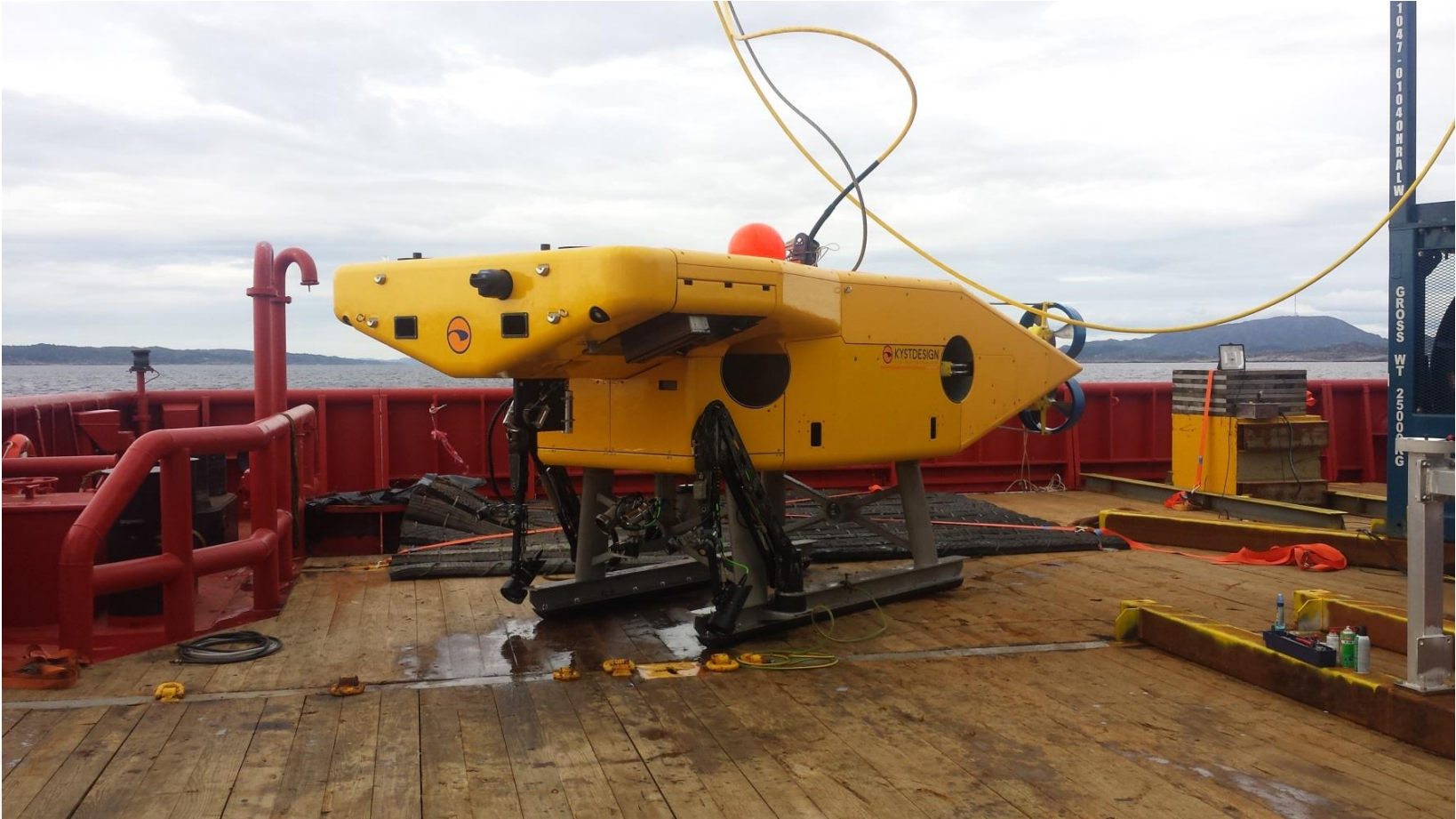
SUPERIOR ROV WITH SKID ATTACHED FOR PIPELINE SURVEY
