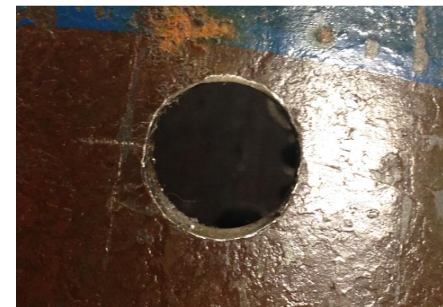
Hole in casing made by the Perforation Drilling Tool
