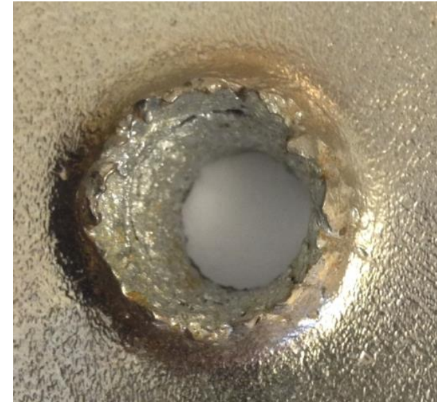
Hole in casing made by Perforation charge
