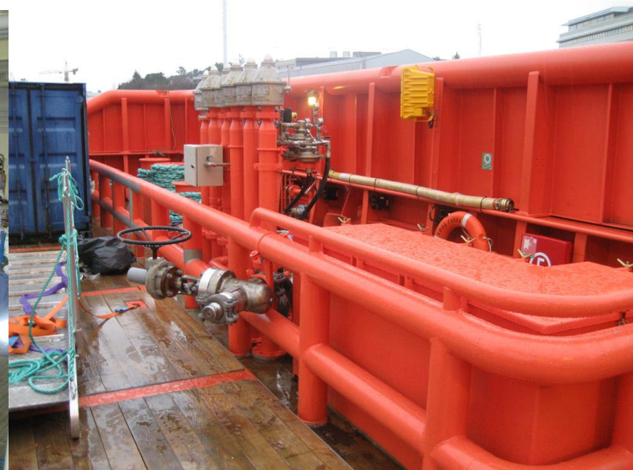
Cargo rail manifold
