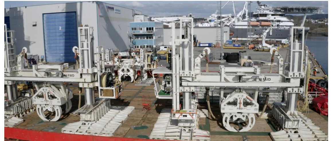
Pipe handling frames
