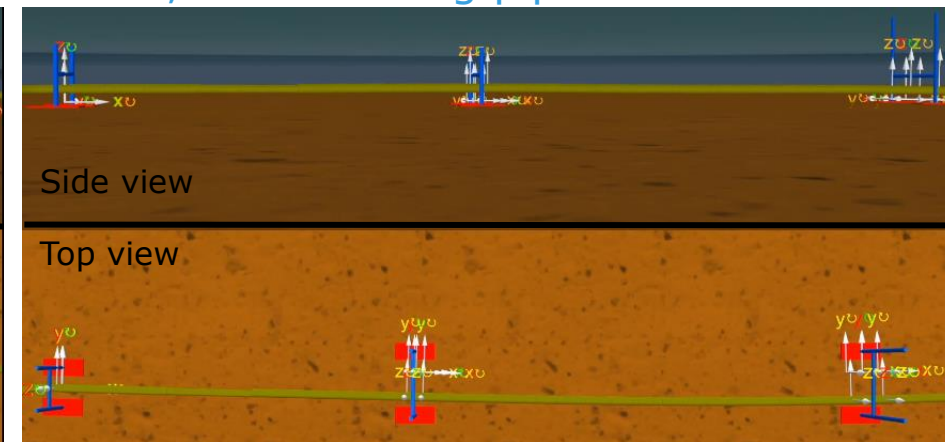
4: Release hog to extend pipeline
