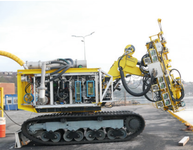
FlexiCore™ system during wet test, deployed from a quay side.
