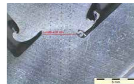
Plug weld, and material testing sample showing fusion line length (red line)
