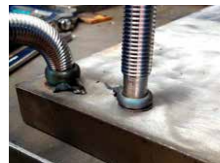
Super Duplex studbolt welds incl bend test
