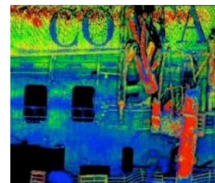
Example of the high resolution subsea laser data acquired on the Costa Concordia.
