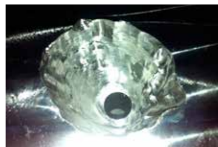
Sectioned test fixture with reproduced crater, and a CNC machined replica
