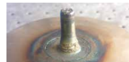
Plug weld, and material testing sample showing fusion line length (red line)
