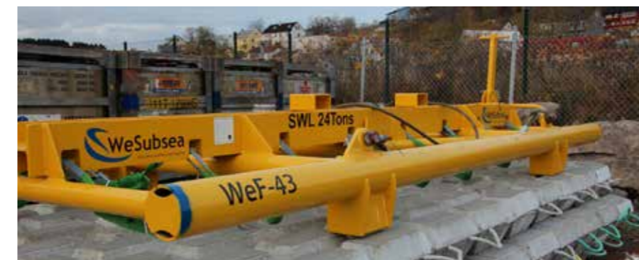
The WeSubsea Lifting Frame for concrete mattresses and our high quality concrete mattresses
