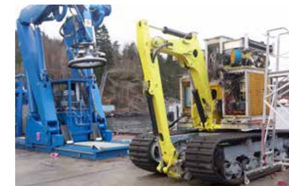
The newly developed Subsea Excavator for dredging and tooling
