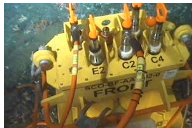
Proserv Open Communication Hub (OCH) for connection of cameras and other instrumentation.
