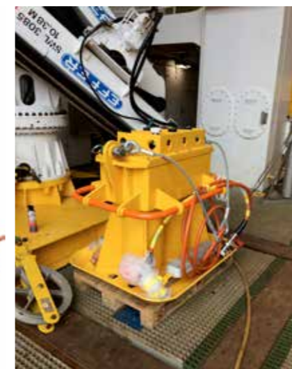
Proserv Open Communication Hub (OCH) ready to be installed subsea.
