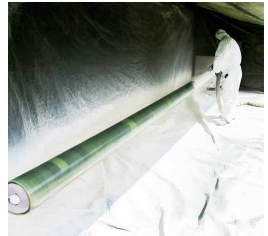
Re-use of TG28/4000 is possible without loss of buoyancy. Here is a 7 meters long floater with green GRP and white PURsub© in production progress.
