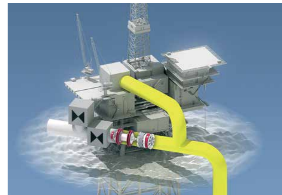
Use of SmartPlug tool technology allows the replacement of topside valves without reducing pipeline pressure or affecting the production of downstream platforms.
