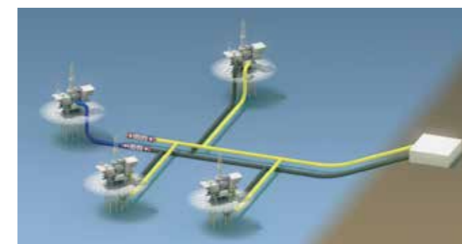
Use of SmartPlug tool technology allows the replacement of topside valves without reducing pipeline pressure or affecting the production of downstream platforms.
