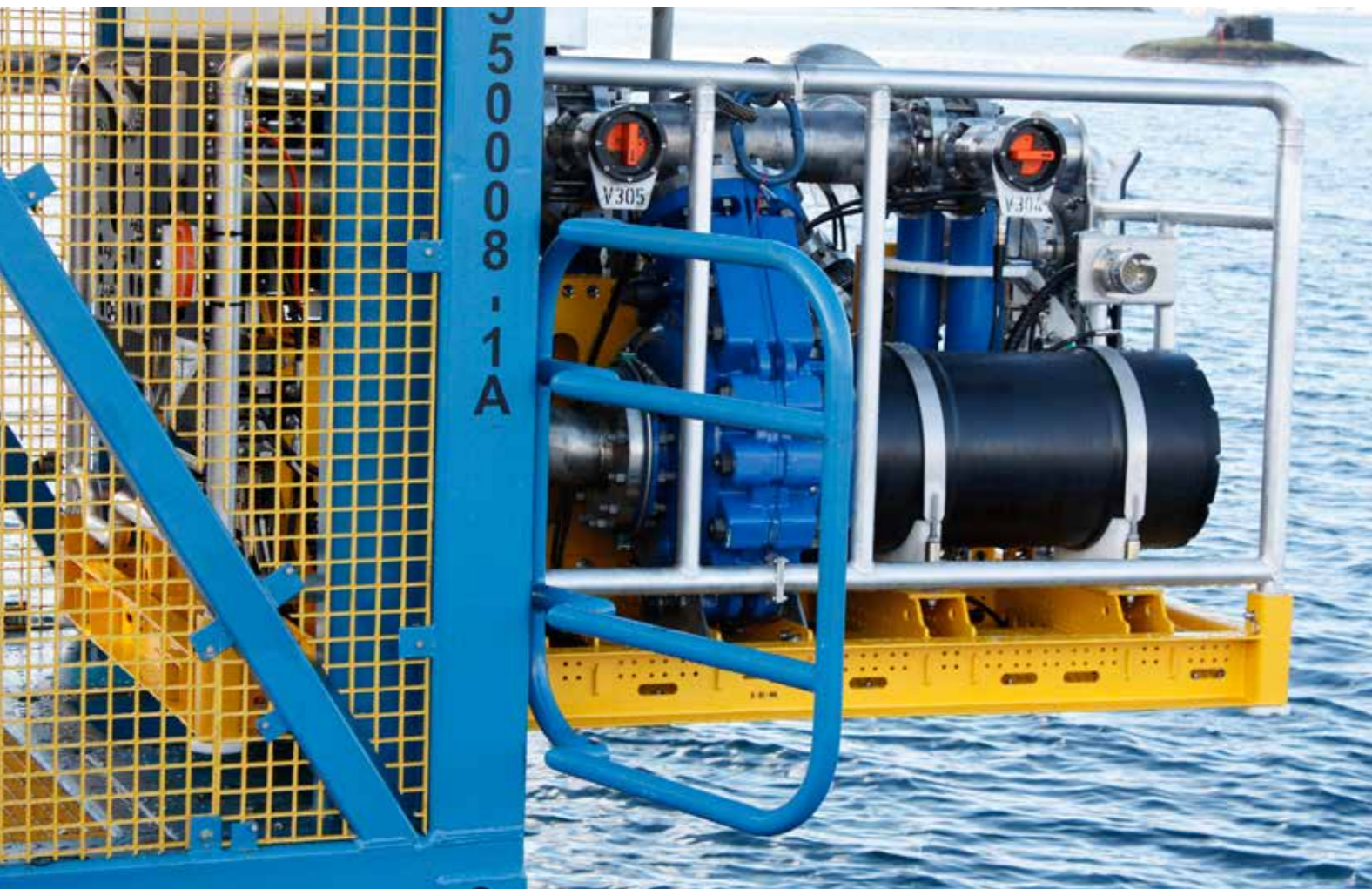
MRR (Mud Recovery without Riser) system med LARS
