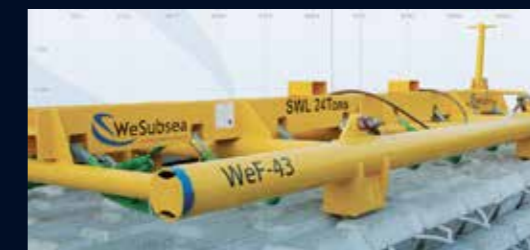
Lifting frame concrete mattresses.
