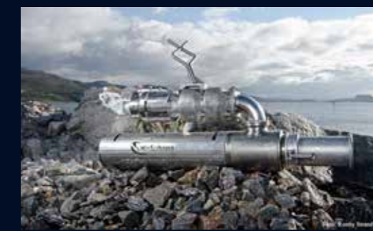
WeSubsea 6 inch ROV dredger.
