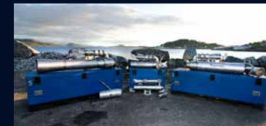
Range of ROV dredgers.
