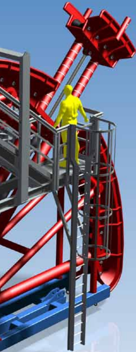
Illustration of new radius controller: Full 3D model and design developed in-house at Subsea7 Stavanger (Above).
