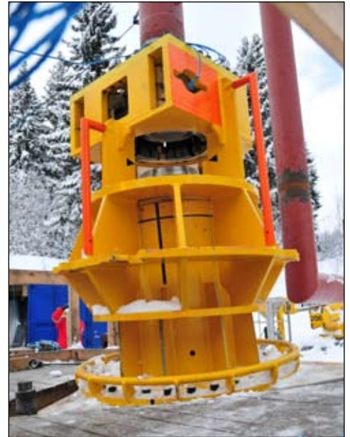
VCS – connector landing, picture from qualification testing
