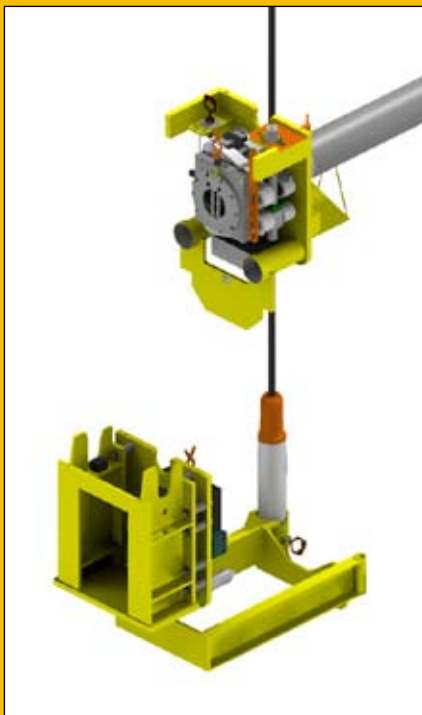
HCS – landing rigid spool using guide wires.
