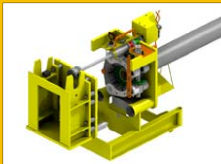
HCS – spool landed, ROV carried stroke tool installed ready for connecting.
