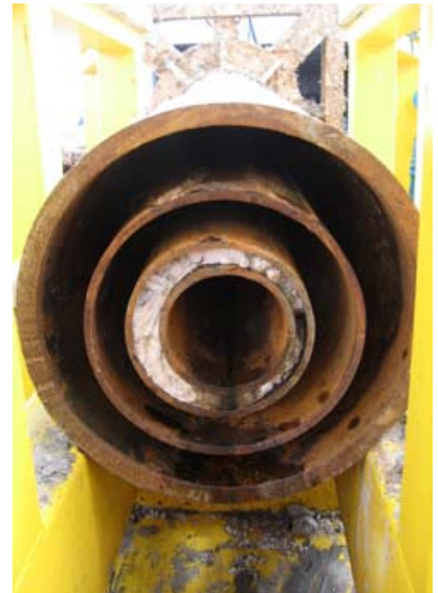
The cut - made by abrasive waterjet cutting
