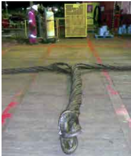
Extreme consequence of heavy steel wire rope after faulty use.
