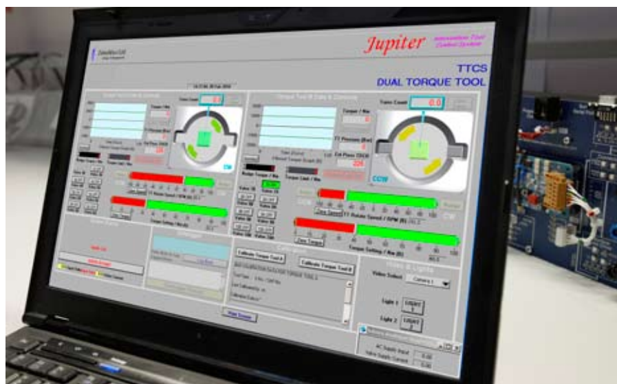
The Jupiter GUI is easily modified by the user for their application; this example shows the simultaneous operation of twin torque tools by a Jupiter 2 Skid Control System.
