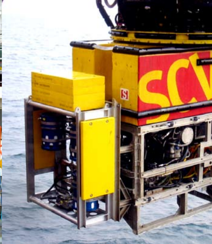
Rear-Mounted IHPU toolskid (Fig. 3)
