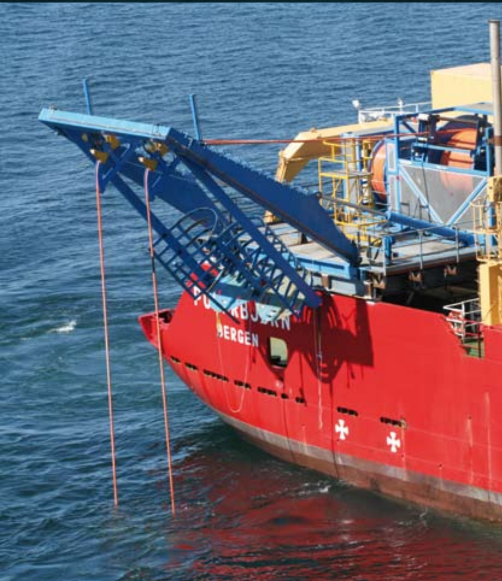
Fig. 3 – Transmitter launching systems
