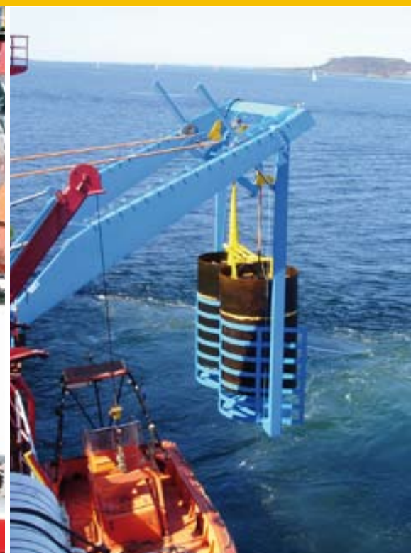
Fig. 2 – Electrodes double-action launching system.
