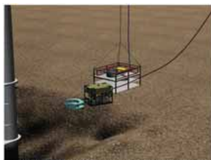
04. WROV transports the GR to the pile
