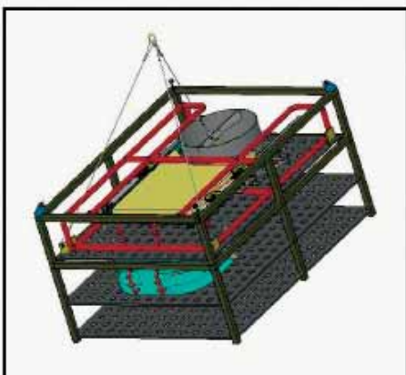
Deployment frame preparation on desk, Step III Assembly ready for DWCM power umbilical connection and deployment sling installation.
