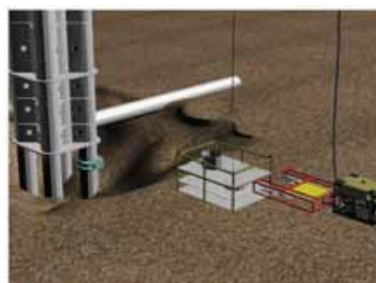
10. WROV removes DWCM from frame
