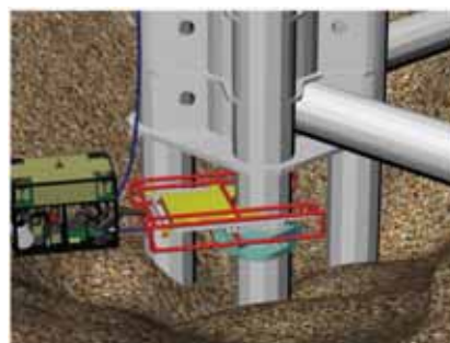
12. DWCM Clamps pile ready to cut
