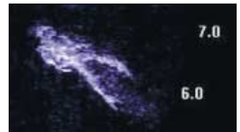
Fig. 3 Image of a diver 6.5 m from the sonar
