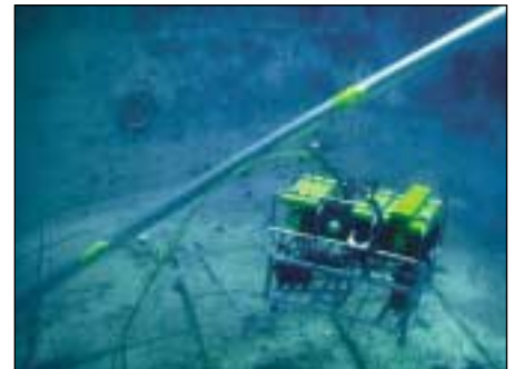
Fig. 7 Leak detection using ROV and DIDSON.
