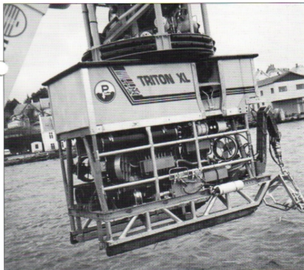
ROSCAN hengende i ROV manipulator.
