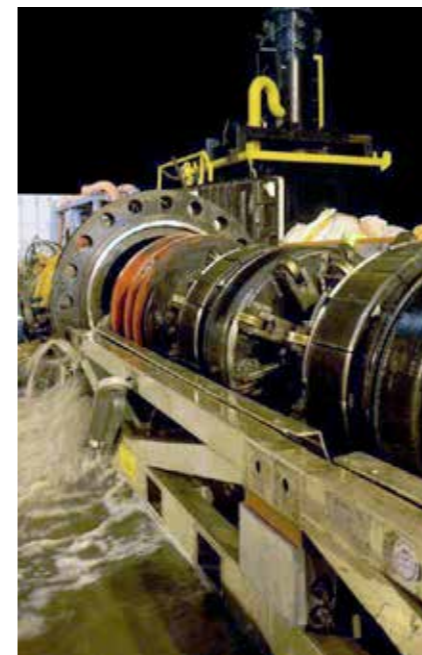
TDW SmartPlug Inline Isolation Tool emerging from launcher receiver.
