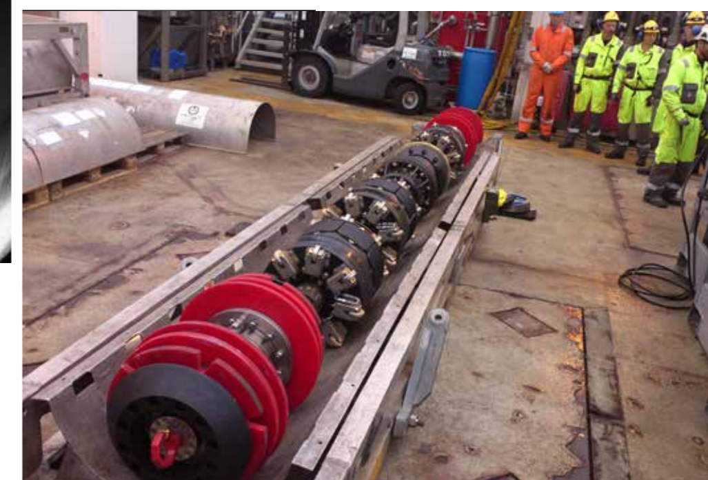
Three-Module SmartPlug® Inline Isolation & Hydrotesting Tool
