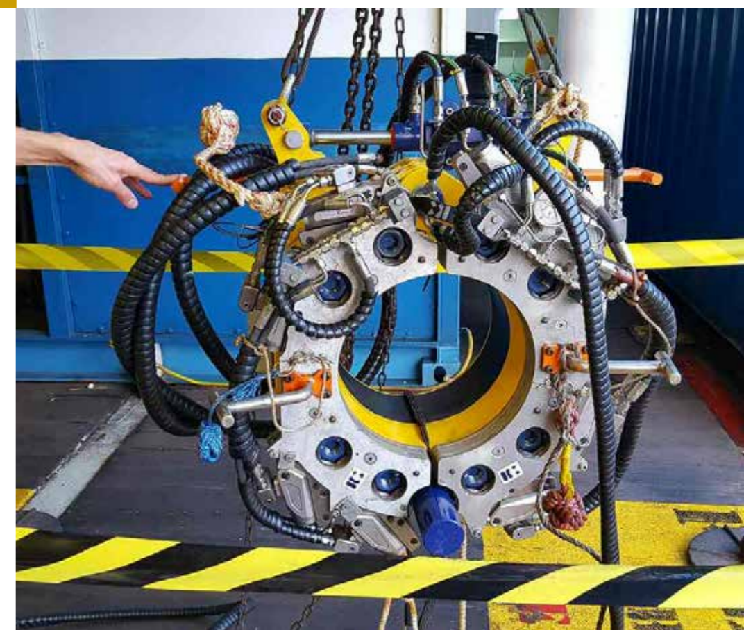
Patch clamp under testing med Torque tools installert.
