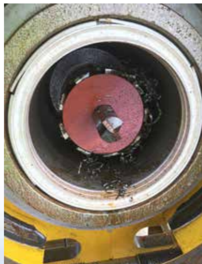
Coupon from Zeepipe IIA in hot tap cutter.
