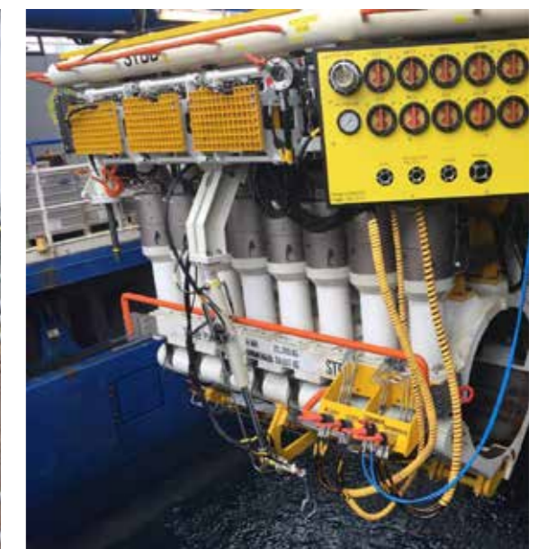
Retrofit tee and installation tool in moonpool of Normand Ocean.
