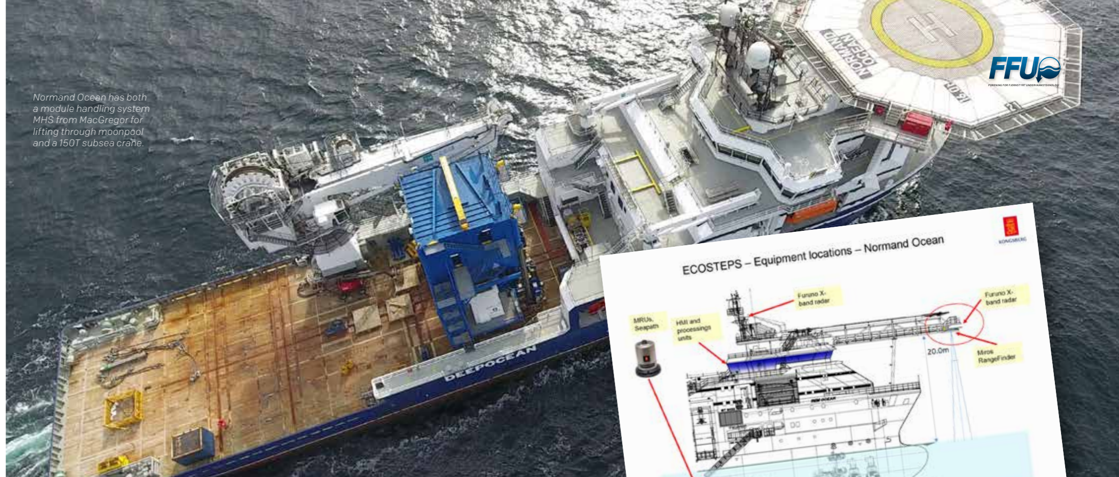
Equipment for full scale measurements on Normand Ocean.
