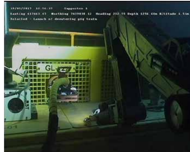
Continuous Valve Operations - ROV Standby with Tool Engaged
