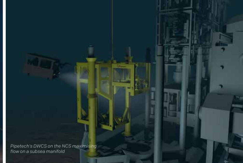
DWCS in action on seabed template ready to remove scale from a produced water manifold
