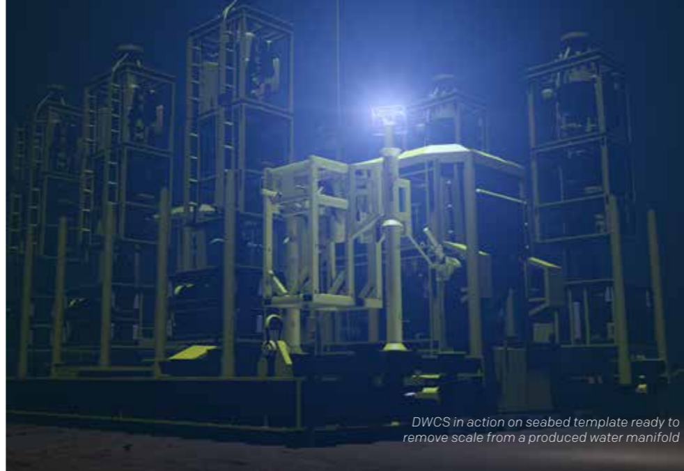
Pipetech's DWCS on the NCS maximising flow on a subsea manifold
