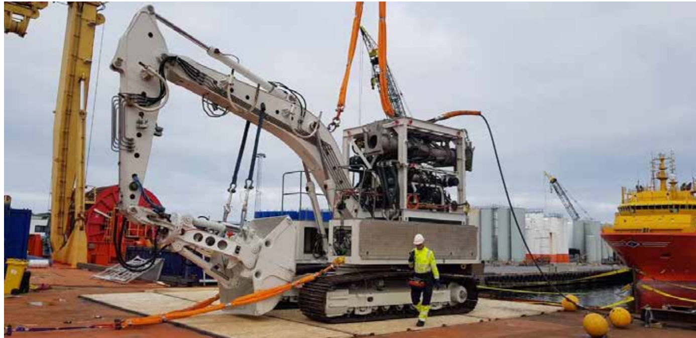
ScanROV is a unique power supply and control unit designed to be used with a variety of tools, here combined with excavator tracks offering a unique combination of mechanical force that that is completely exceptional. Here with a 2 m3 grab, which can easily be replaced with levelling bucket, Diamond Wire SAW or ejector.
