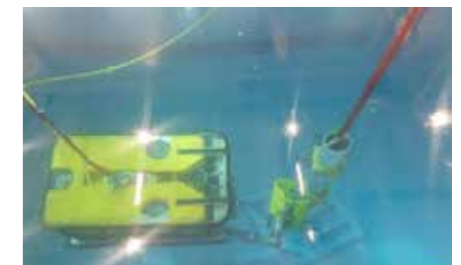
Full scale wet testing of tooling and method with WROV in a large pool
