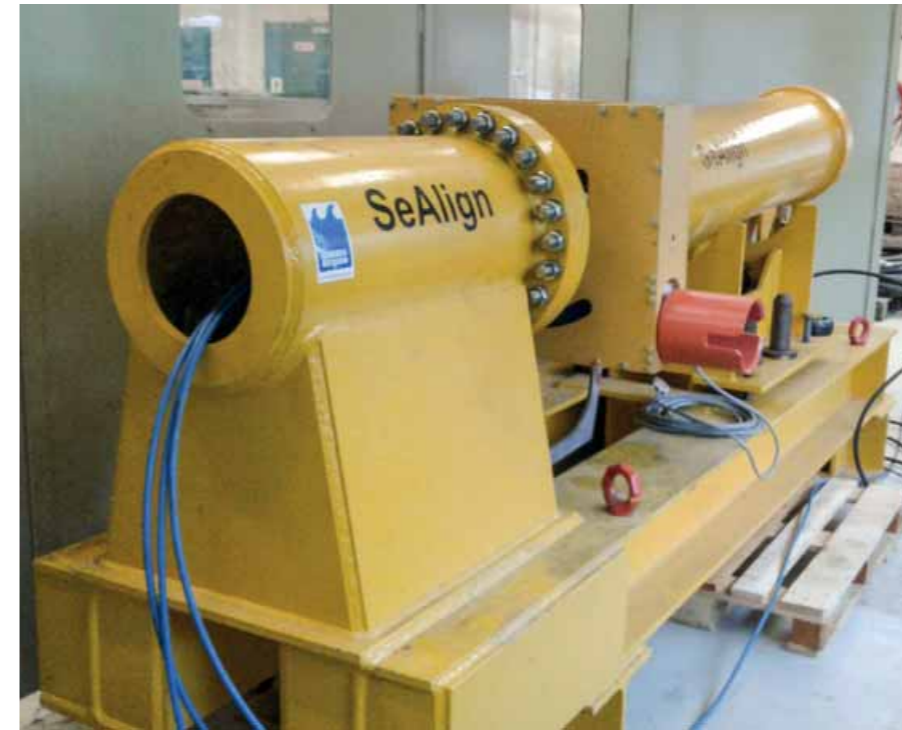
6" SeAlign connector during cyclic sliding test
