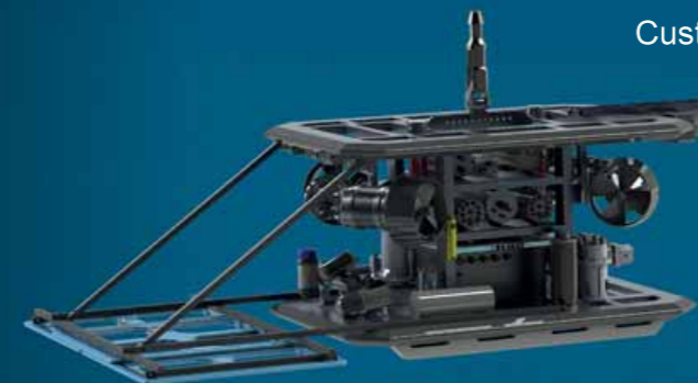
Argus Rover up to 3000msw depth rated
