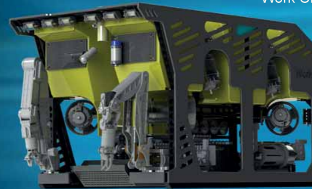
Argus Worker up to 7000msw depth rated Proven with more than 4000 hrs at 5800m
