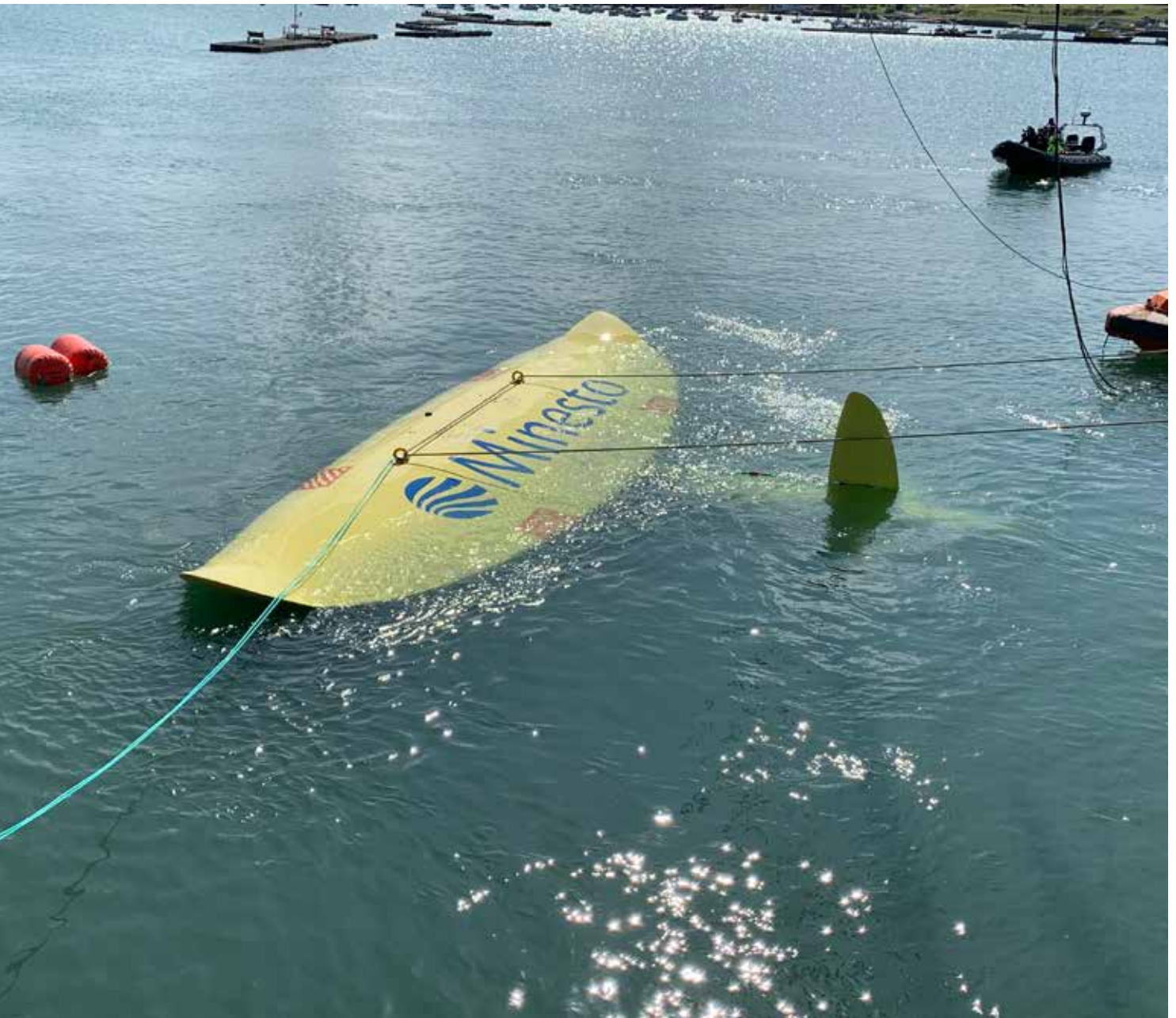
Minesto's utility-scale marine energy converter DG500 during commissioning trials in North Wales. The DG500 has a rated power of 500kW and a wingspan of 12 meter.
