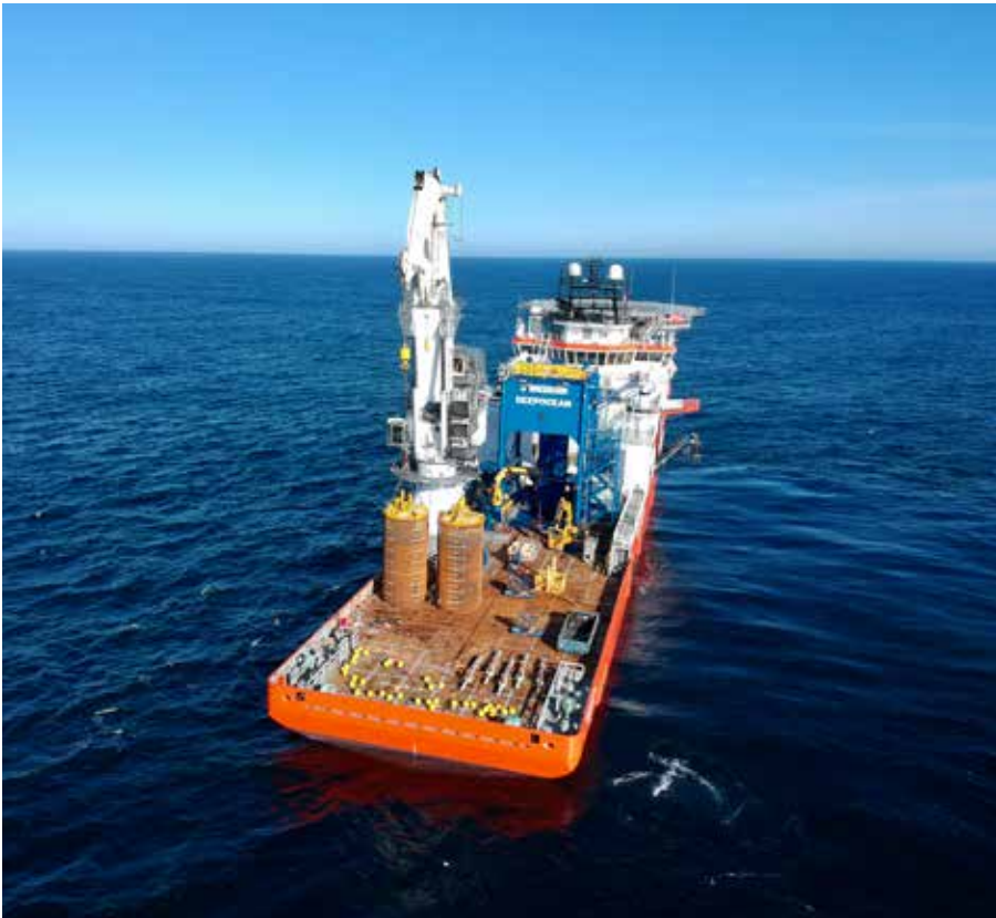
Normand Ocean has both a subsea offshore crane, and a MHS module handling system from MacGregor
