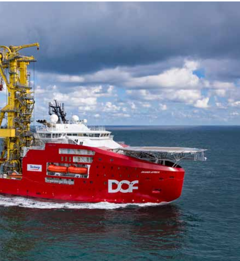
construction vessels. Even the subsea crane has a lifting capacity of 900 Tons.
