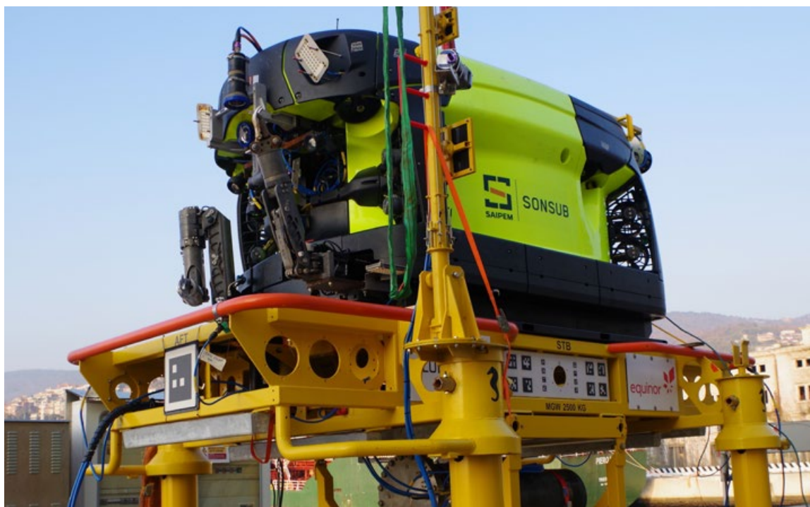
Hydrone-R UID on Equinor's Subsea Docking Station
