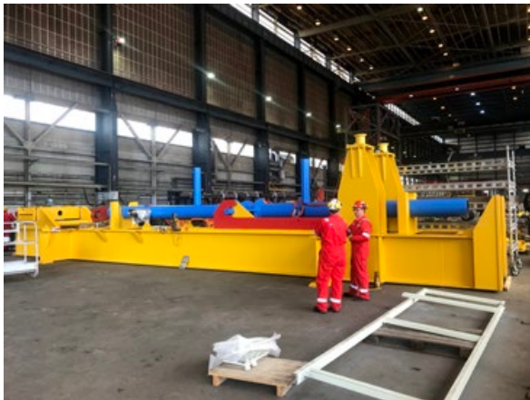
In-line Manifold under testing. Rosenberg Worley, Stavanger.
