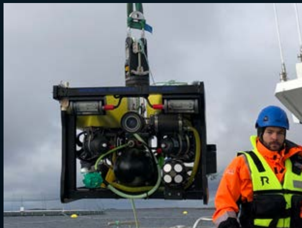
SINTEF ACE RoboticLab: Autonomous underwater operations with an ROV equipped with state-of-the-art sensors. Photo: SINTEF/Eleni Kelasidi
