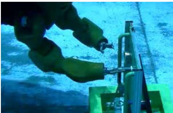
An image from a scene of Aquanaut executing an autonomous mission. Insert EFL Connector.
