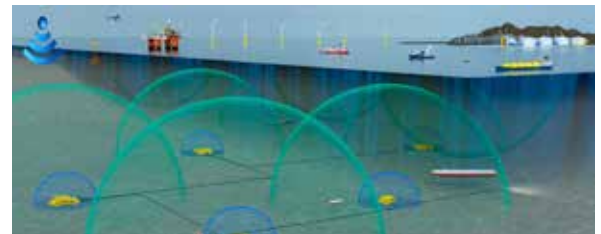
Figure 6 Equinor 3-modal communication concept for UIDs, inductive (yellow), optical (blue), and acoustic (green). Image courtesy of Equinor.
