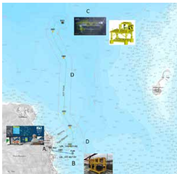
Figure 1 Trondheim's OceanLab: A - Shoreside control room; B - Subsea location 1 (PLM module); C - Subsea location 2 (SDS module); D - Umbilical.
