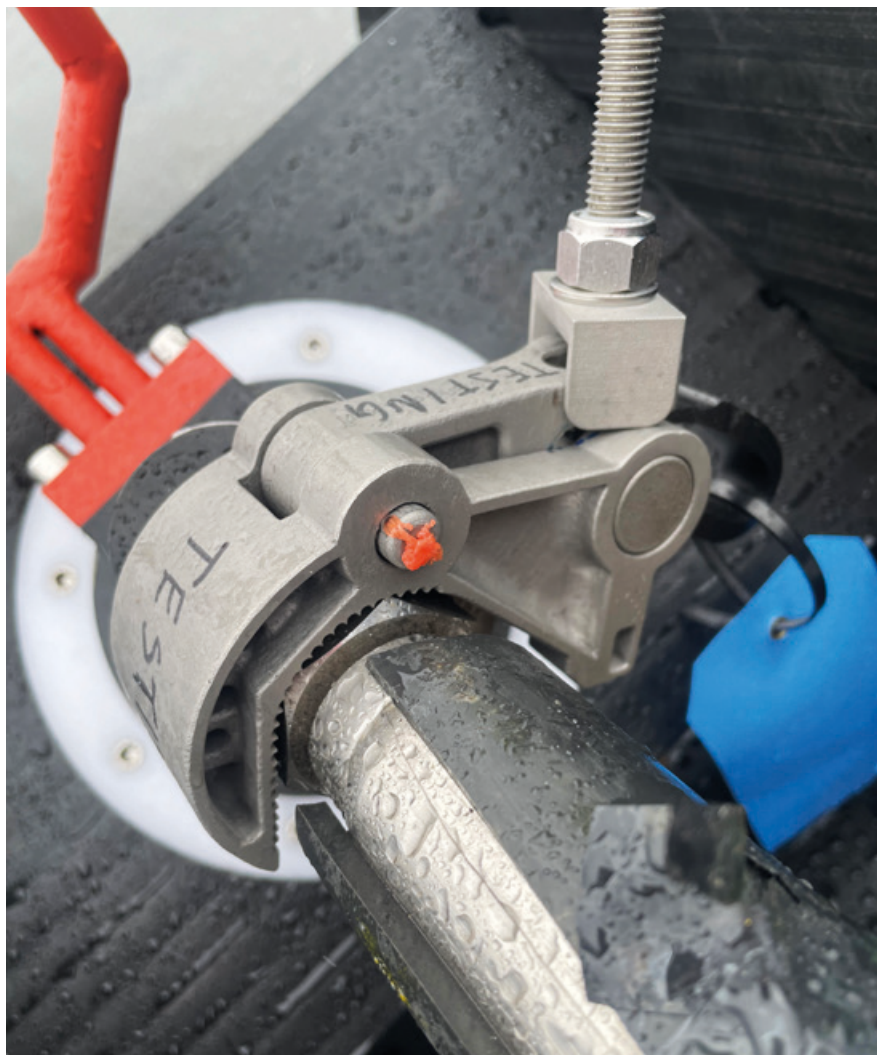
Metal 3D printed clamp during SIT.
